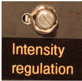
Fig.13 Intensity regulator potentiometer on the back panel (optional).
