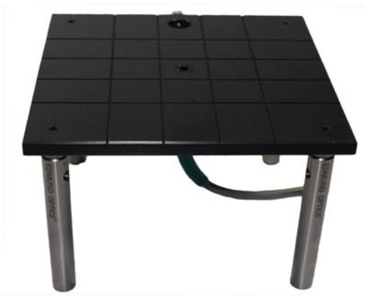
Fig. 14 Face-down configuration. Reflectance probe (SMA terminated) is attached to a adapter under the table. Light shines up and the sample should be place face-down on the table.
