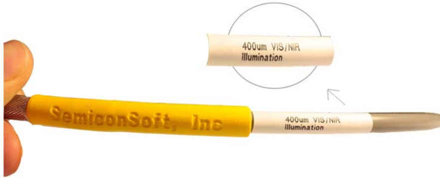
Fig. 11. Illumination leg marking of reflectance probe
