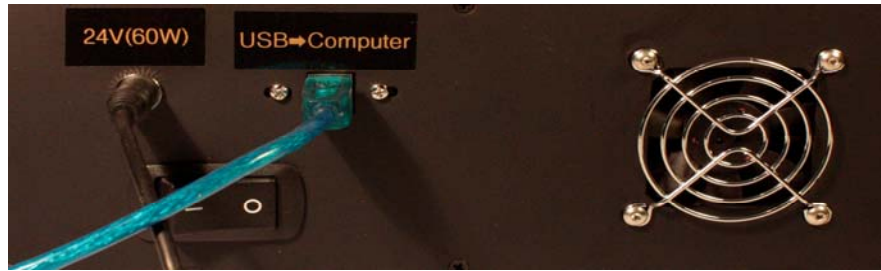
Fig. 3 Back panel of MProbe UVVis/UVVISNIR system with USB cable and power adapter connected
