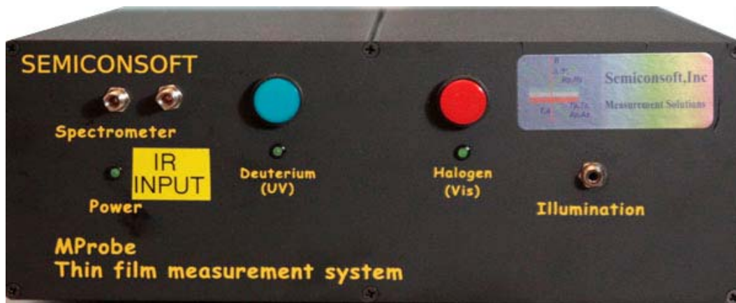
Fig. 7 The front panel of MProbe UVVisNIR system. Notice two separate spectrometer inputs: use Yellow coded end of reflectance probe for IR channel (Green for UVVis channel)
