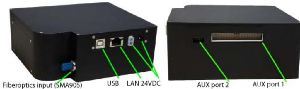
Fig. 2 Ariel spectrometer Footprint: 144mm x 130mm, Height: 55mm
