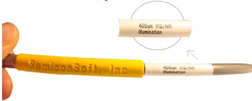
Fig. 8. Illumination leg marking of reflectance probe
