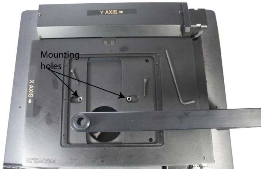
**Fig. 3.** Stage mounting holes are accessible, after stage is moved and can be lined-up with the threaded holes in stage post.
