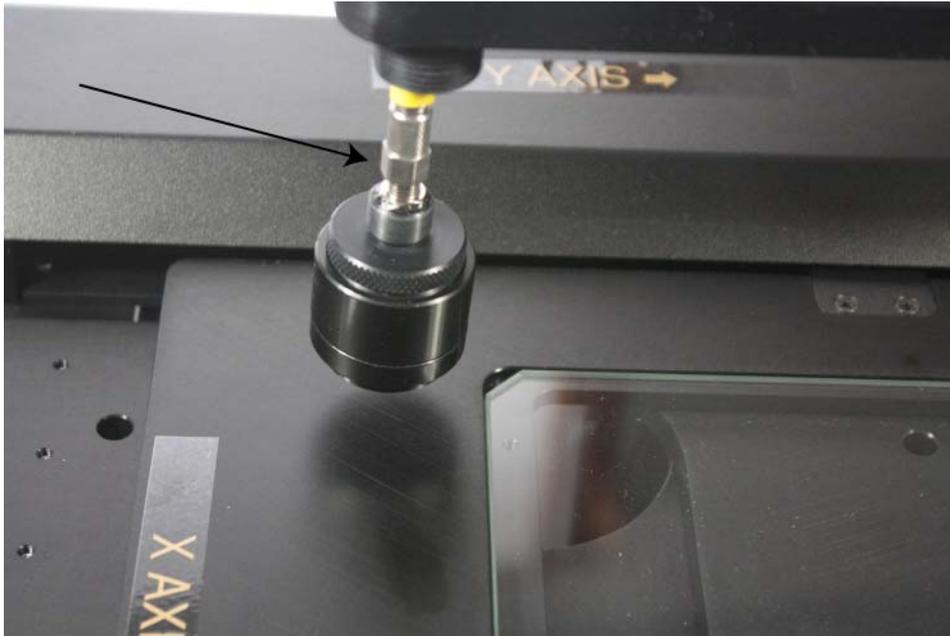
Fig.5. Put reflectance probe thru the hole in the holder and attach it to the SMA connector on the lens. Do not connect other ends to the MProbe system yet...
