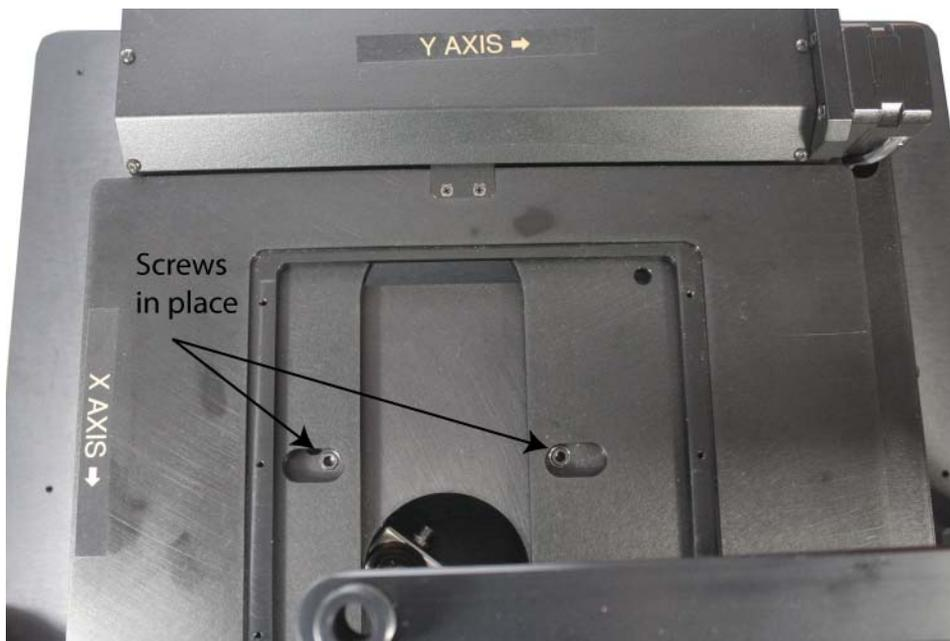
**Fig. 4.** Stage is mounted using two 8-32 screw (do NOT tighten the screws fully) before other 2 screws are inserted.
